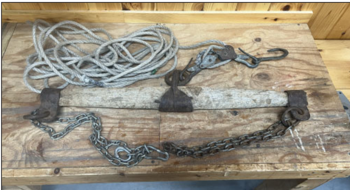
This is a block and tackle with an old yoke used for spreader. Short chains on either end with snap links are used to secure legs to spreader. Cut between tendon and bone on each hindquarter and attach chains. A long 2x with an eye bolt lagged across the bottom of a few trusses on which to attach the block and tackle. Block and tackle attached to the ceiling can be adjusted to the height of the deer to allow for skinning and dividing into quarters. Photo by Gregg Schefferly.
