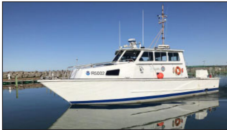
The team utilized NOAA's Great Lakes Environmental Research Lab's RV Storm, a 50-foot research vessel equipped with a multibeam sonar and dedicated to research within the sanctuary. Photo courtesy of NOAA.
