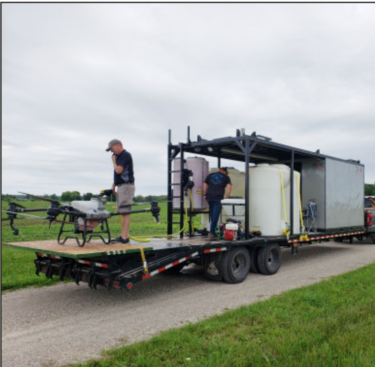
Drones operated by Eagle Endeavors Drone Service based in Monroe, Mich., spray herbicide by drone on Bob Leonard's soybean field in Harrisville. Leonard said the crop would have been lost because the heavy amounts of rain made the perfect environment for weeds to grow and left the ground too wet and muddy to drive in traditional weed-suppressing spraying machinery. Alan Peters (front) and Brandon Kantz operate the drones. Courtesy photo.
