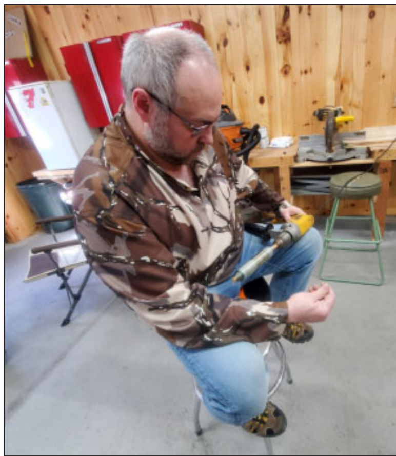
Gregg demonstrates using a half inch wood dowel on a cordless drill to remove fishing line from reels.
