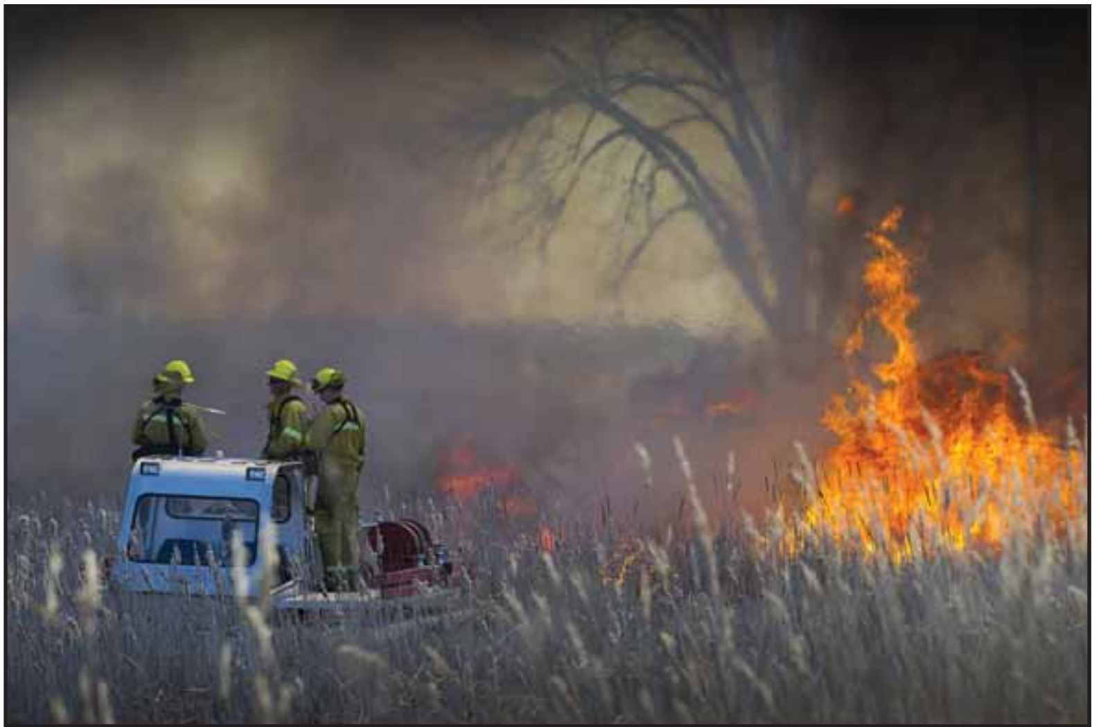
DNR fire officers monitor a prescribed burn (for habitat improvement) at Fish Point State Game Area, Bay County, from the deck of a “Marsh Master” – a tracked vehicle that floats and allows transportation into wetland areas. Photo courtesy of Michigan DNR.
