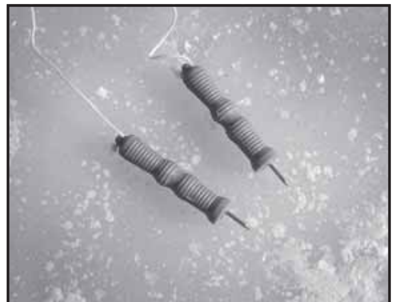
A pair of ice spikes, like these, can help someone who falls through the ice get back on top of it.
