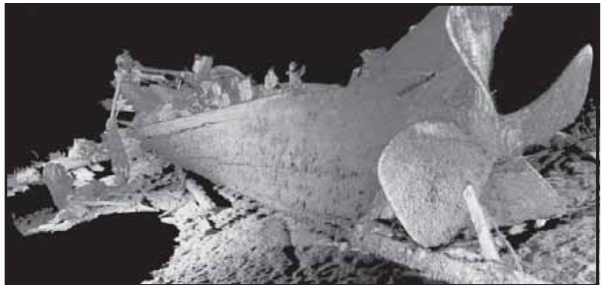
A laser is used to map the wreck of the Monohansett in Lake Huron. Graphic courtesy of Sarah Waters, Thunder Bay National Marine Sanctuary.
