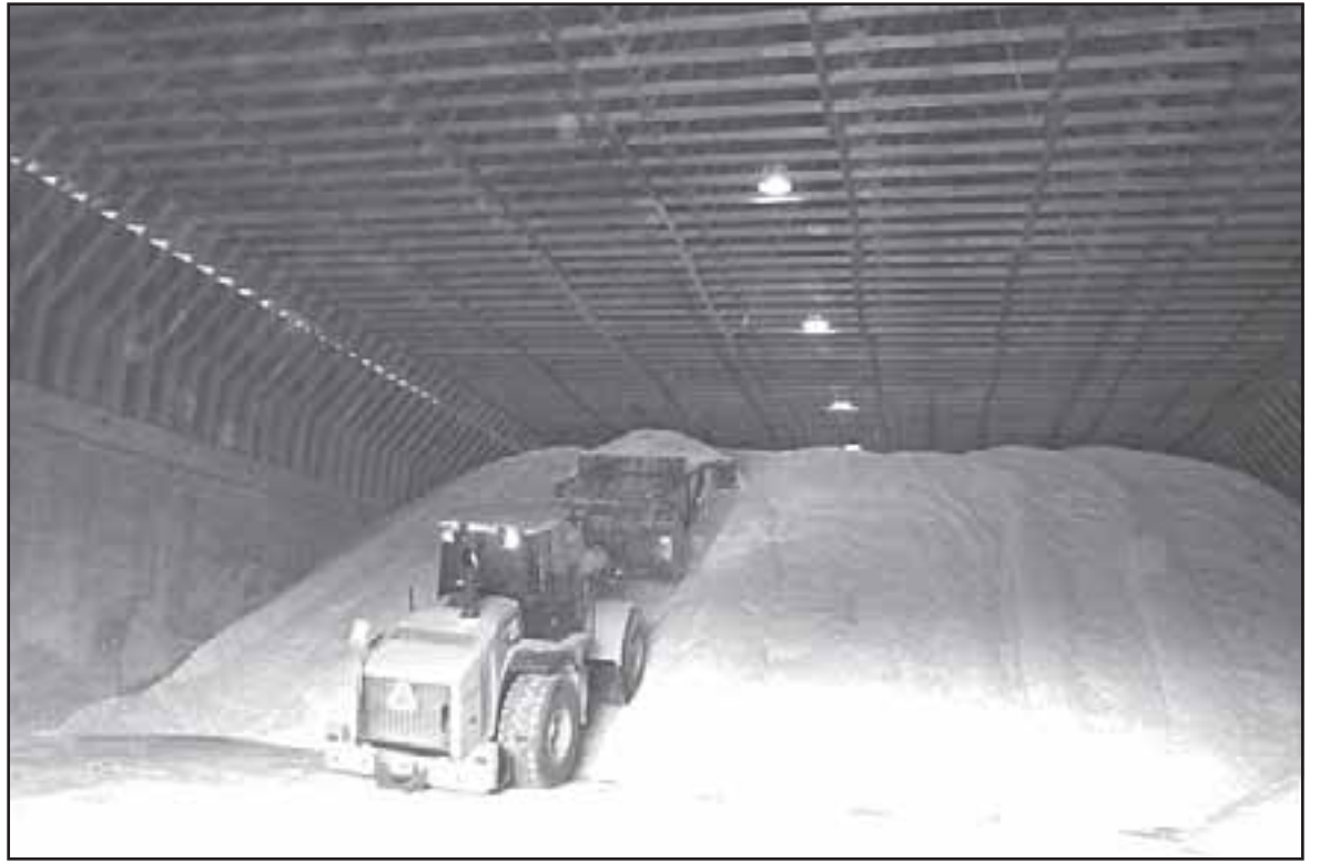
A special extension blade on a wheeled loader aids in stacking salt up to maximize the space in the Alcona County Road Commission's salt storage facility. Courtesy photo.
